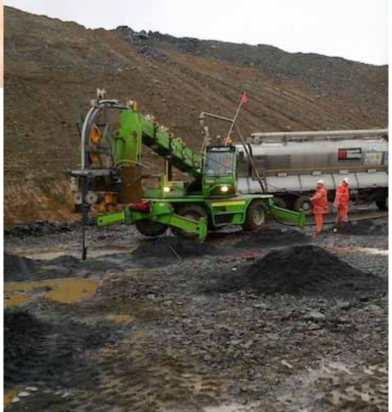
Above: The Merlo Remote Explosive Loading Unit
