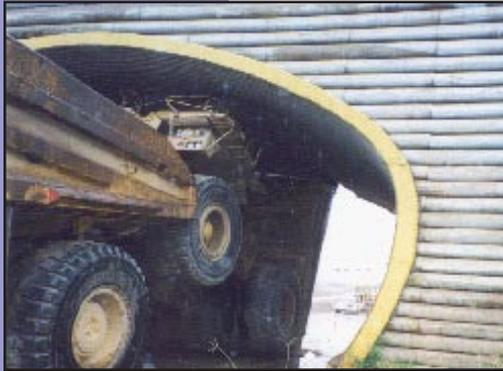
DRIVER'S cab jammed against underpass. Crushed handrails, second truck used to stabilise elevated truck
